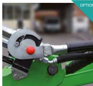
Hydraulic quick coupling for compact loaders
