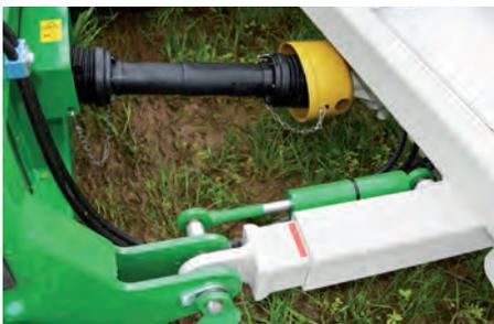
Direct drive – transmission on transfer shaft
