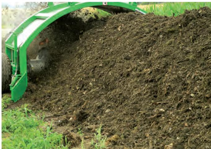
With the TG 301 a successful composting is achieved easily and quickly. This is due largely to the turning axis that works perfectly and that moves the material from the inside to the outside.
