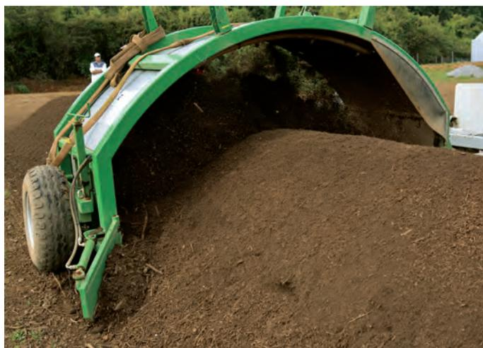
The TG 301 is a compost turner that is easy to use, mechanically operated, stable and maneuverable with optimal weight distribution. It is ideal for field-edge composting, small composting plants and organic farms with compost production up to 6,000 tons per year.
