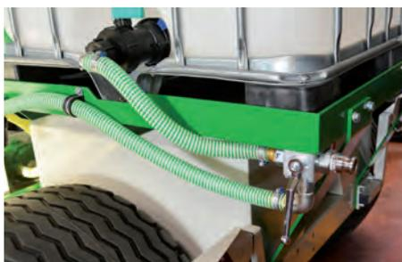
External water intake possibility for external water sources
