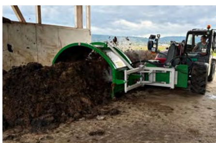
Maximum pile size: 2.5 x 1.2 m, enabling aerobic composting.
