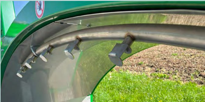
Water spray bar with 4 impact plates – enquire about irrigation options
