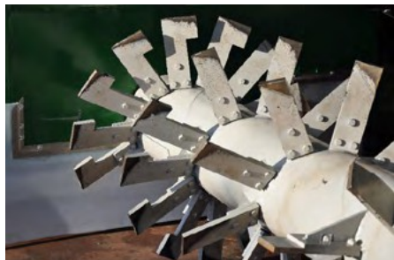
A good turning shaft works the material from the inside out. Gentle turning allows the microorganisms to multiply optimally throughout.
