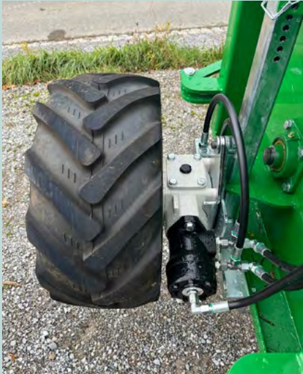
Hydraulic drive wheel with automatic control.
