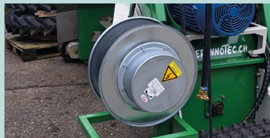
Cable reel up to 80 m for water hose or electric cable reel.
