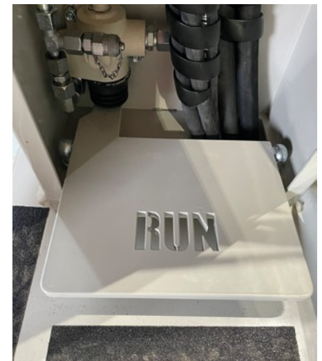
Emergency stop pedal without electrical installation.
