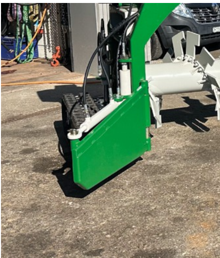
Hydraulic feed blade on right and left, even with electric drive. (Load sensing hydraulic pump)
