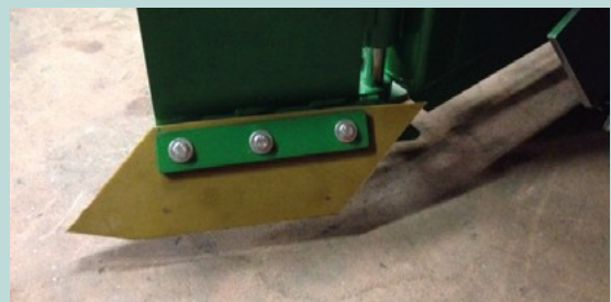
Rubber on the feed plates (for paved areas)
