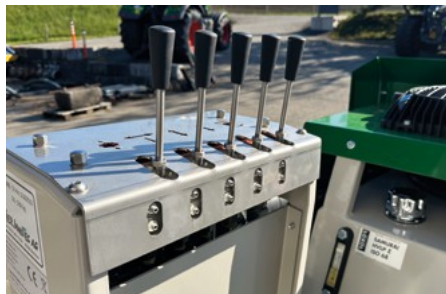
Drive lever control is held in the set position.
