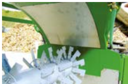
All wear plates are made of chromed steel.
