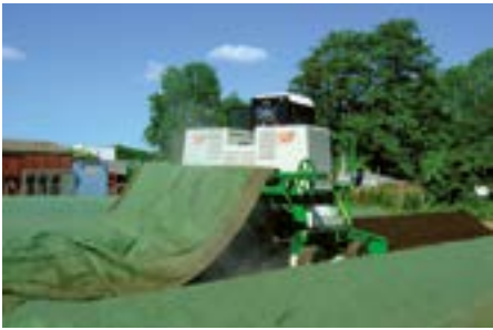
Fleece roller hydraulically height-adjustable with quick-change system
