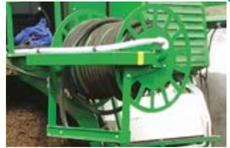
Hose reel with automatic hose guide. Winds hoses in-and-out up to 80 meters.
