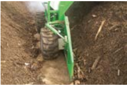
Single swiveling, hydraulic shields ensure clean troughs.
