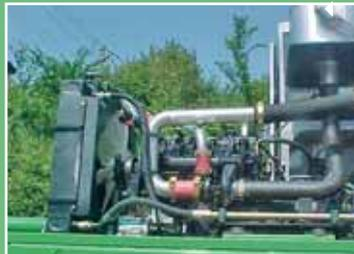
The vibration buffer (silent blocks) between chassis and engine-frame reduces noise to a minimum.
